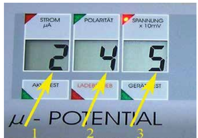
Fig. 3. Potentiometric indices of healthy people (indicated by arrows: 1 – current strength, 2 – electrical conductivity of oral fluid; 3 – potential difference, the last index should be multiplied by 10)
